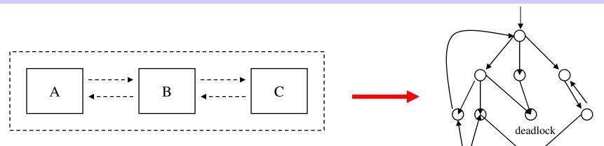
Each component is modeled by a FSM.
