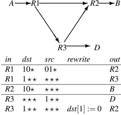
Figure 1:  $R1$  has a QoS routing rule that routes packets from a video source on the short route and other packets to destination  $1**$  along a longer path that traverses  $R3$ .  $R3$  has an ACL that drops packets from  $1**$ .  $R3$  also rewrites the middle bit in  $dst$  to 0. This ensures that re-routed packets reach  $B$  regardless of the value of  $dst[1]$ .
